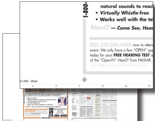
Ink key values can be imaged directly onto the plate making setup even simpler.
